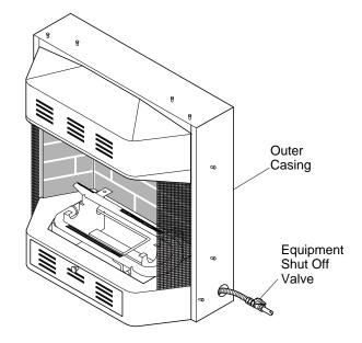
Figure 21 - Routing Flexible Gas Line
